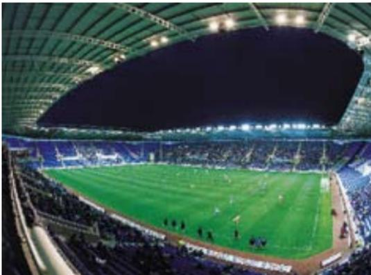
A football stadium lit using Mundial floodlights. The luminaires are mounted along the roof of the stand down two sides of the pitch, and a mix of light distributions is used to correctly illuminate all the playing area. Lighting levels for television are supplied by ensuring good levels of vertical illumination in the camera directions.
